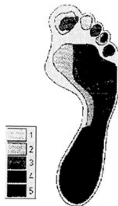
Fig. 2.20. A drawing showing the pressure distribution under the right foot of a subject standing motionless on a stiff surface. The drawing is based on visual estimation of areas of equal density shown by a photograph of a planar track. The differently coloured areas correspond to different ranges of pressure of the foot/surface interaction; the pressure grows with the increasing index of the colour pattern.
